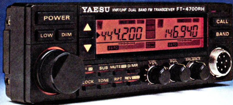
FT-4700RH control head (1 15 / 16 " x 5 7 / 8 " x 1")
